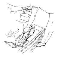
8. Firmly grasp the belt midway between the clutches and pull upward and rearward to remove. See illustration.
